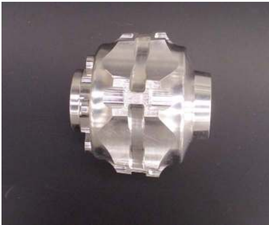
Figure 34 – Forged wheel-hub with no treatment.
