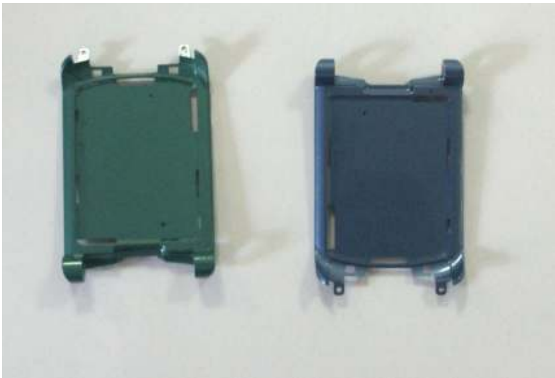
Figure 39 – Part of cell phone case after anodising and powder coating (22)
