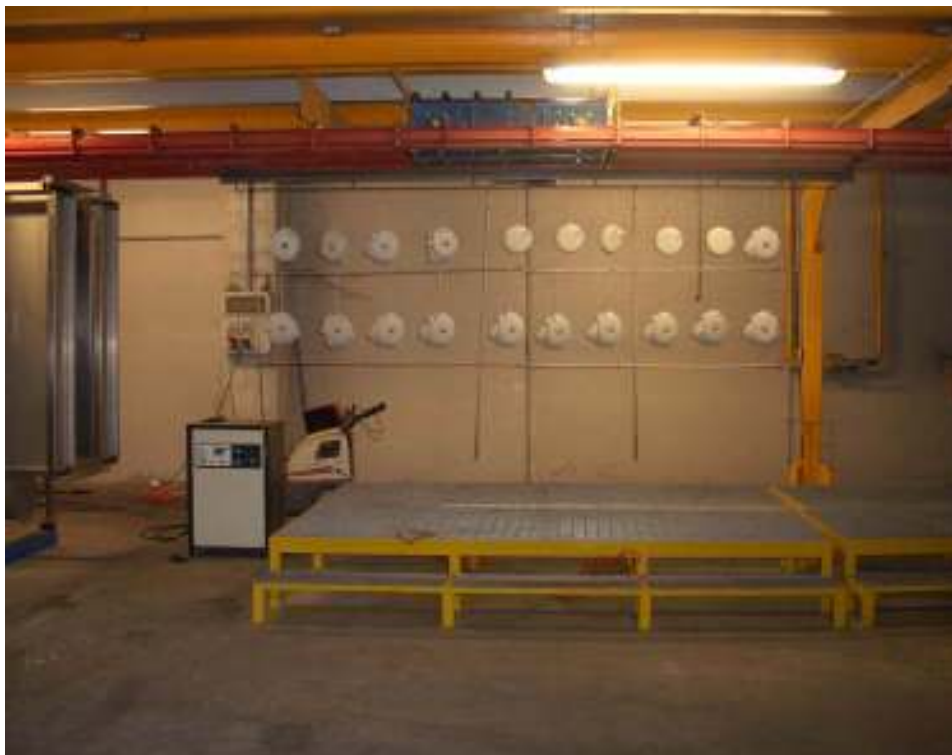
Figure 28 – Anodised pieces ready to enter the powder coating booth, (on the left) and subsequently to the curing oven (on the top)
