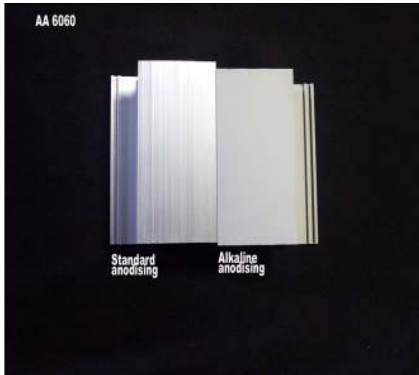
Figure 43- Comparison of AA 6060 aluminium alloy after conventional and alkaline anodising
