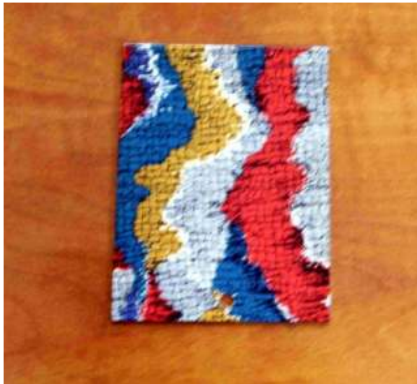
Figure 41 – Special decorative finishing produces by sublimation on anodised magnesium. In this way any plain of fantasy coloration is possible. (Italfinish proprietary process)
