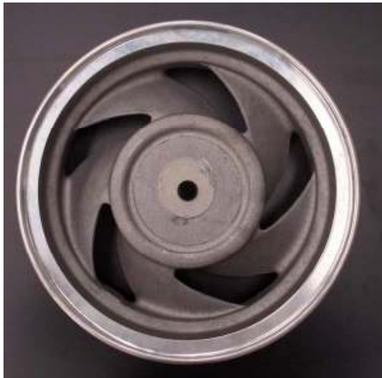
Figure 6 – Scooter wheel (22) The opaque part is blasted and the remaining one is machined.
