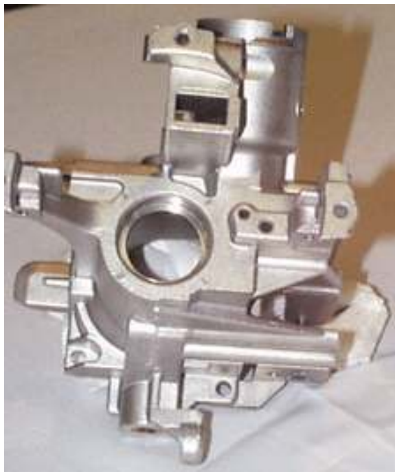
Figure 2 – Steer column box (Ford), weighing only 340 grams (15)
