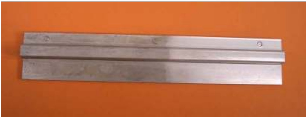
Figure 22 – Examples of magnesium extrusion partly etched in acid solution for 15 second (right part) (22)
