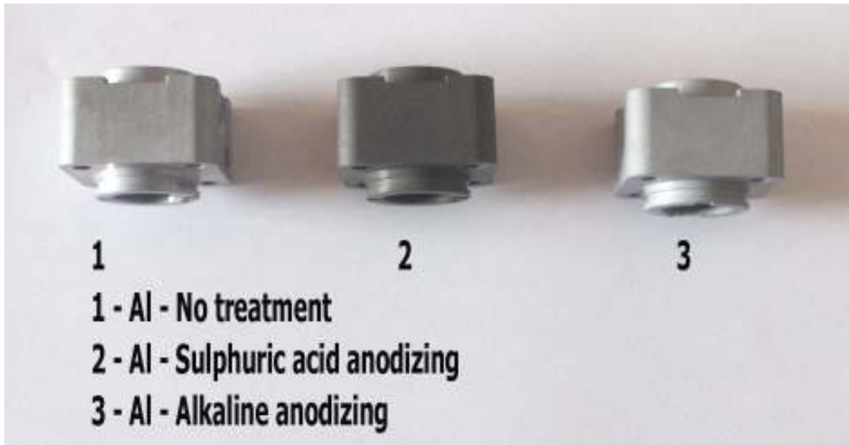
Figure 42 – AlSi12 die-cast alloy anodised aluminium
