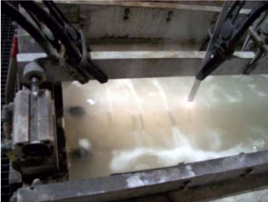
Figure 21 – Micro-arc or spark anodising process performed on Italfinish pilot plant
