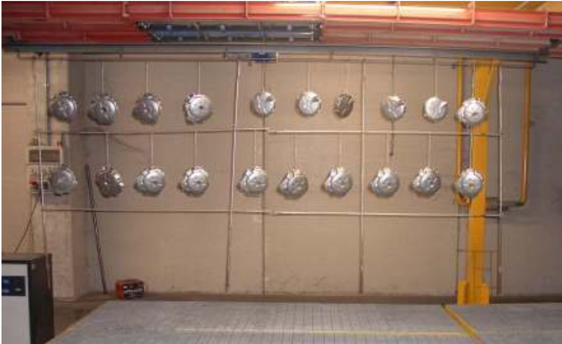
Figure 29 – The powder coated pieces after the curing oven (on the top)
