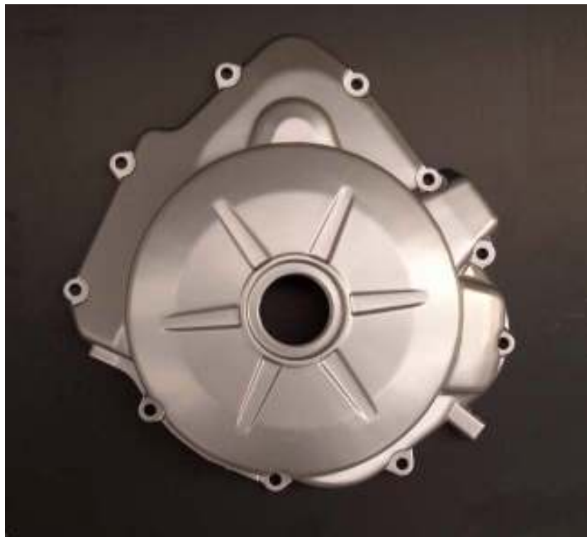
Figure 30 – One of the pieces after powder coating and ready to package. The sample is same type of figure 23, and no evidence remained of the previous superficial problems.
