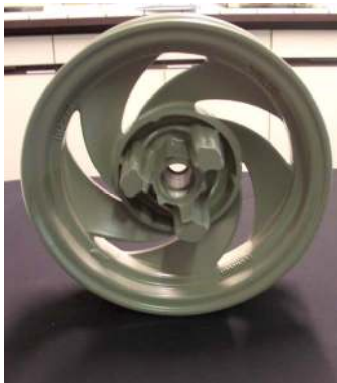
Figure 32 – Scooter wheel after anodising and epoxy base coat by DuPont. The additional coats will be added by the final customer later.
