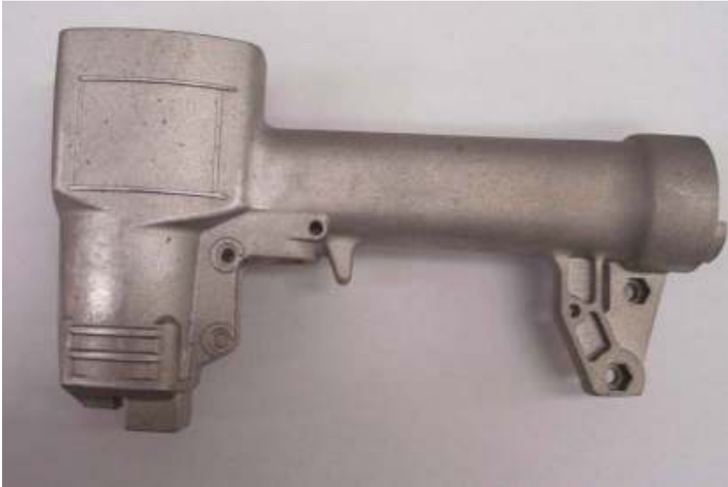
Figure 5 – Nailer casing (22). The piece arrived blasted with evident corrosion pits.
