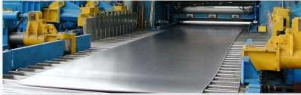
Figure 11 –Rolling magnesium roller (24).
