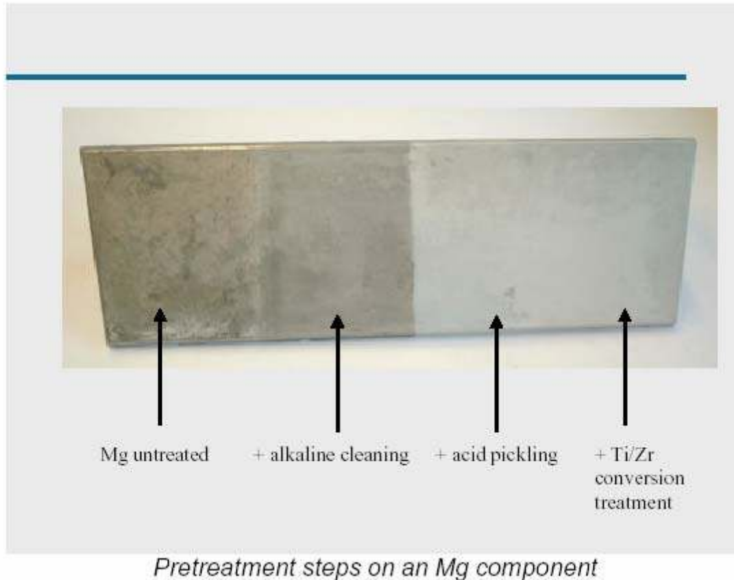
Figure 12- Conversion coating on magnesium (29)
