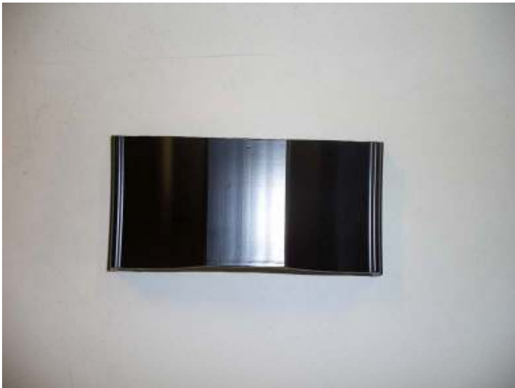
Figure 36 – Forged wheel part after anodising and ED paint (BASF)
