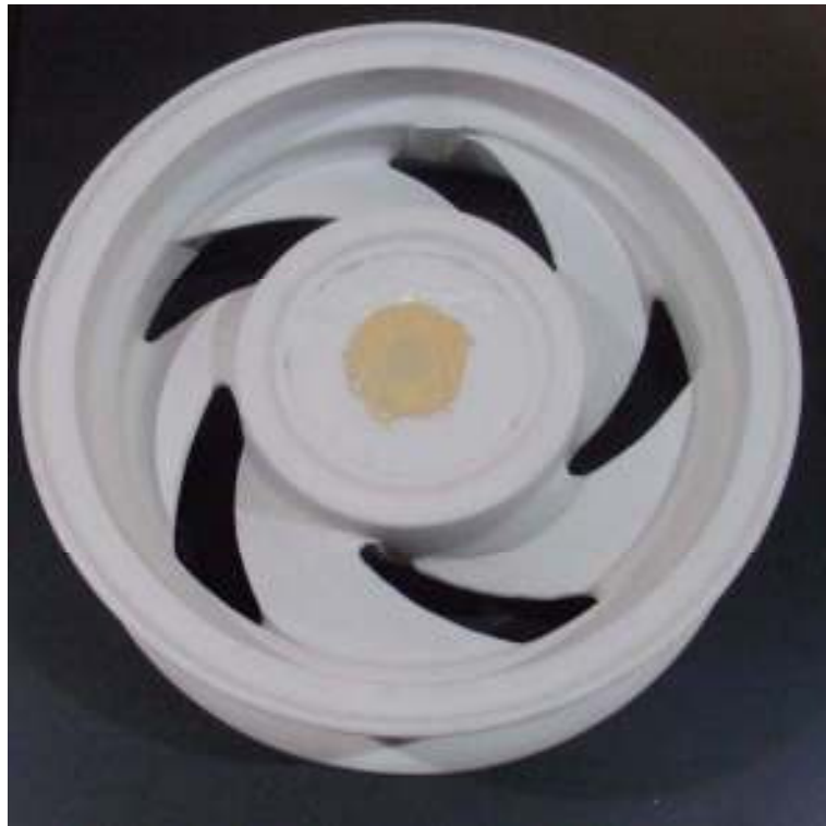
Figure 31 - Scooter wheel after anodising (similar item of figure 6) (22). The brown plastic tape has been used to cover a mild steel insert present in the sample we received.
